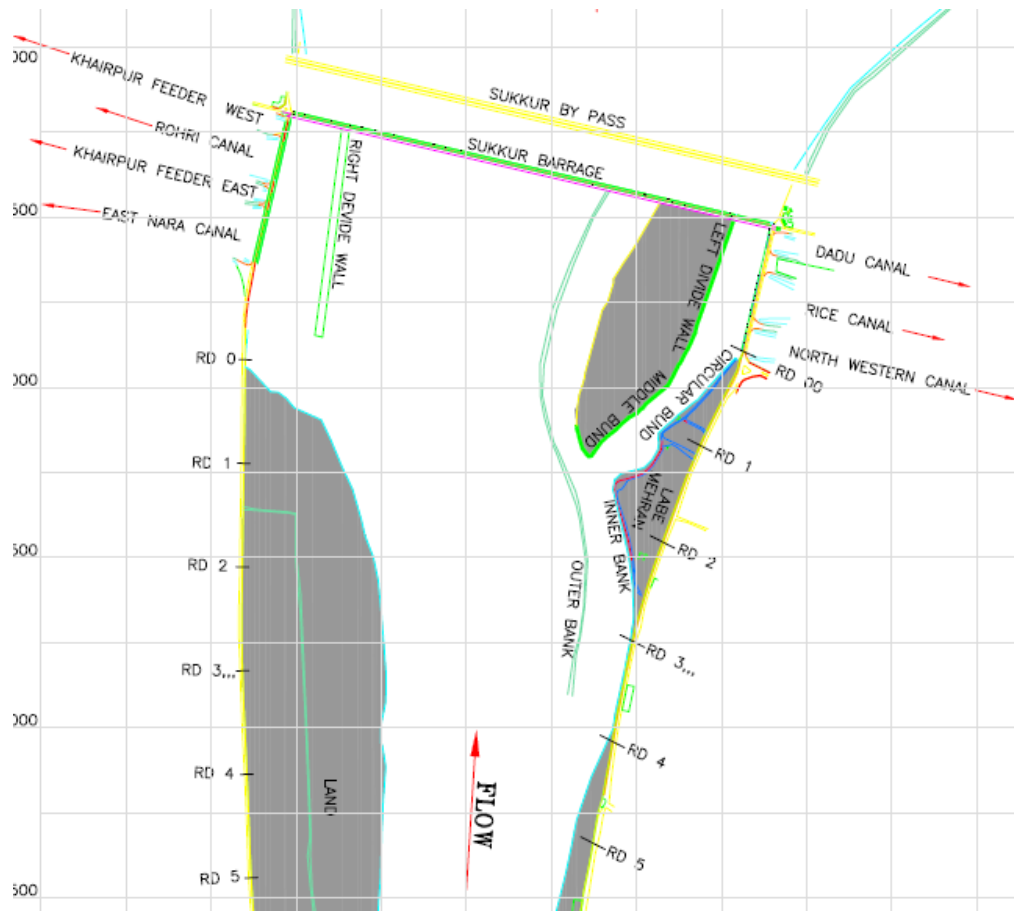
Figure 8. Layout of Sukkur Barrage and Off-take Canals
